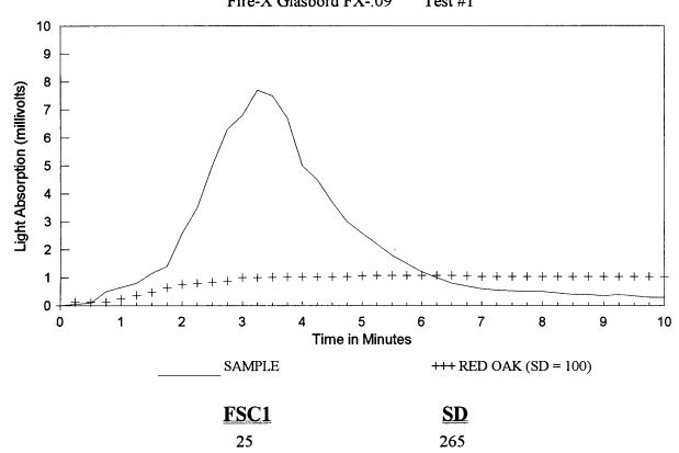
CAN/ULC-S102 Surface Burning Characteristics of Fire-X Glasbord FX-.09"
